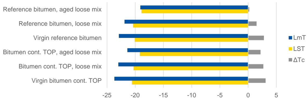
Figure 2. Analysis of 70/100 reference bitumen and 70/100 bitumen containing TOP by Bending Beam Rheometer
