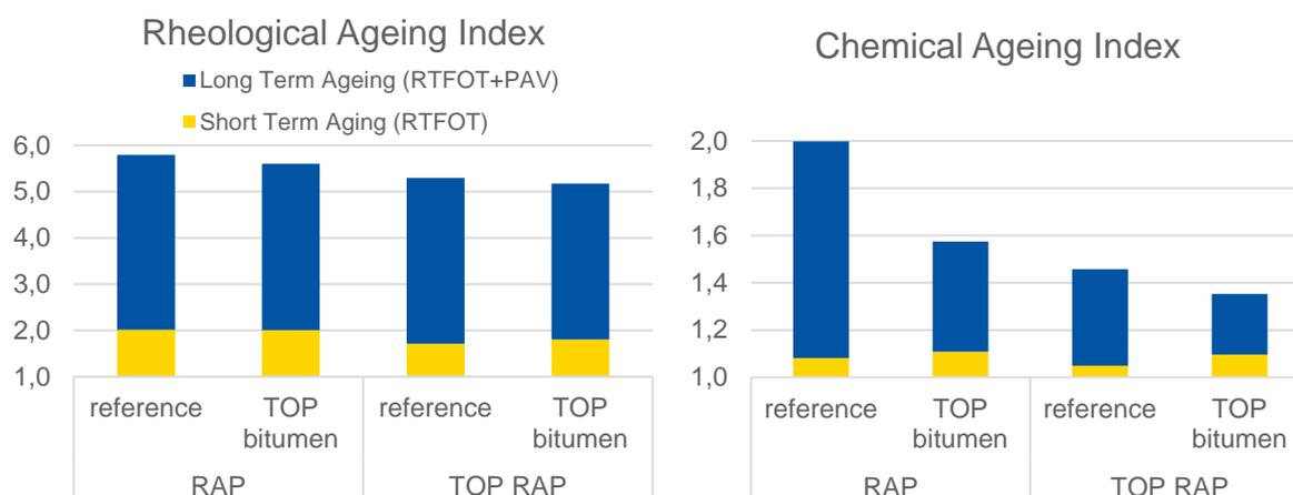
Figure 4. Rheological and Chemical Ageing Index of bitumen with and without TOP in RAP with and without TOP
